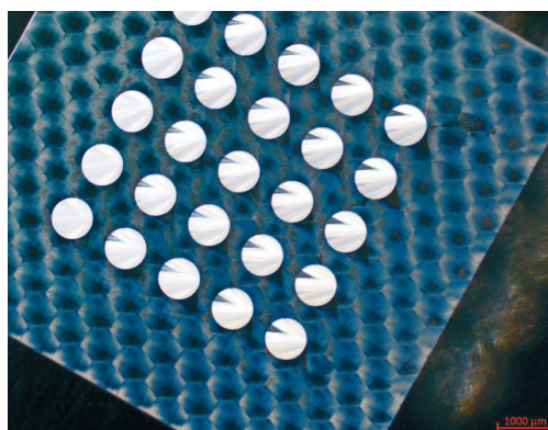
PDMS stamp, bottom view, with conical cavities. This disposable print tool is made on your lab bench.
